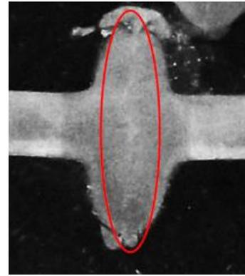
Figure 7. Optical Micrographs of macro section of Flash Butt Welding. White line indicates the decarburized zone.
