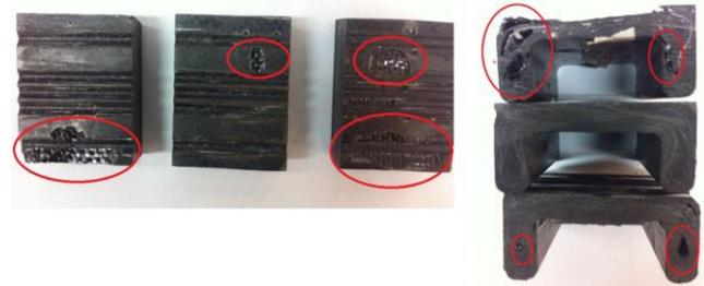
Fig. 10. Defects obtained in first prototypes of clamps with a fiber/matrix ratio of 60/40. Left: lack of fiber and resin around the grooves for the screws. Right: voids inside the clamps.
