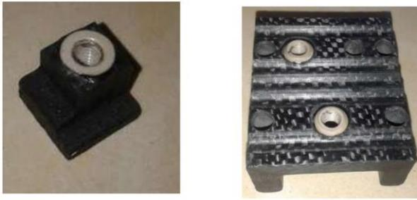
Fig. 13. Machined pieces with PEEK inserts. Left: wedge. Right: clamp.
