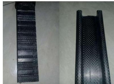
Fig. 11. Defect free clamps obtained by increasing the fiber-resin ratio to 70/30 in weight.
