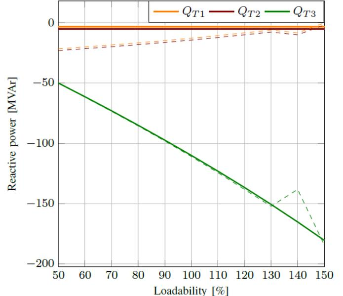
Fig. 7. Transformers reactive power (—with STATCOM; ---without STATCOM).
