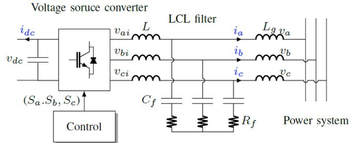
Fig. 2. STATCOM device diagram.
