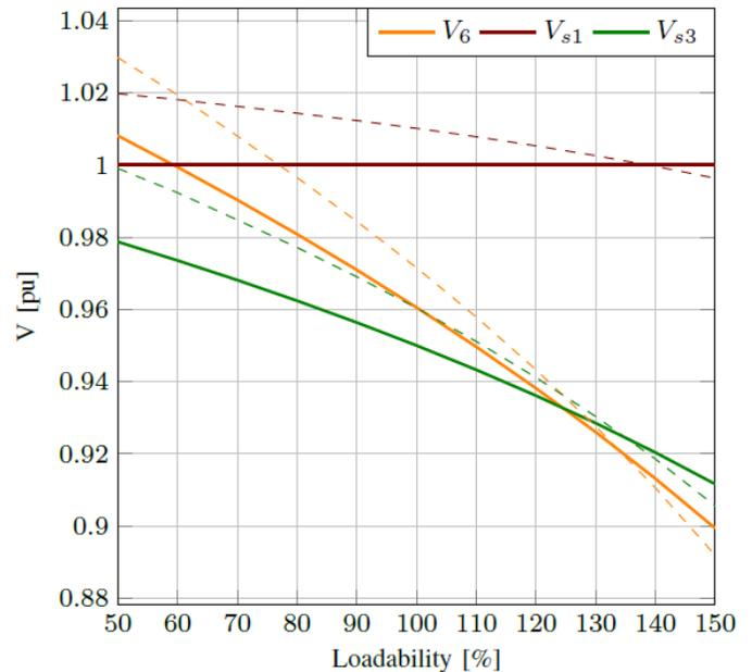
Fig. 5. Voltages of the representative nodes (—with STATCOM; ---without STATCOM).
