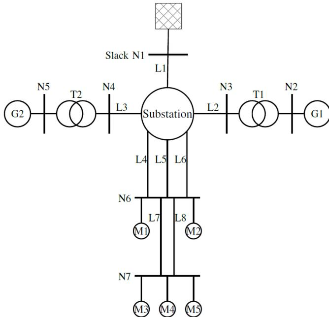
Fig. 3. Power test system with an electrical substation 500 kV/110 kV.
