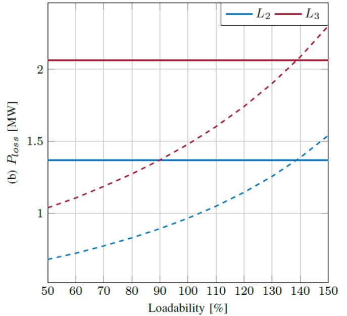
Fig. 6. Transmission lines power losses (—with STATCOM; ---without STATCOM).
