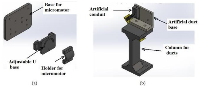
Fig. 10 (a) Design of the endodontic motor base (b) Design of the artificial root canal base
