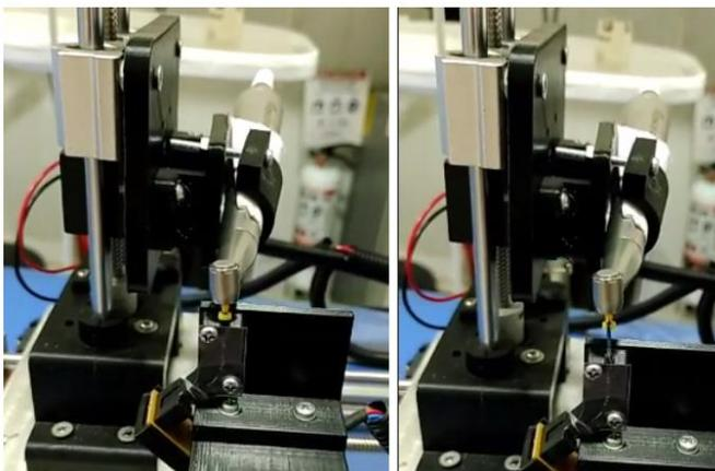
Fig. 12 Dynamic test on Azdent® F1 brand file
