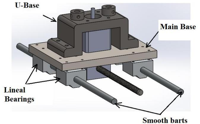
Fig. 9 Design of the main base module
