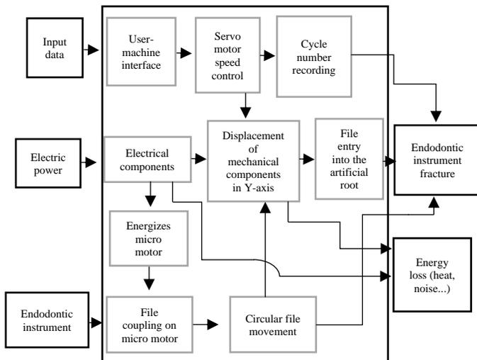
Fig. 5 Clear box for the test bench
